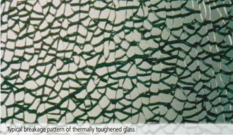
Typical breakage pattern of thermally toughened glass
